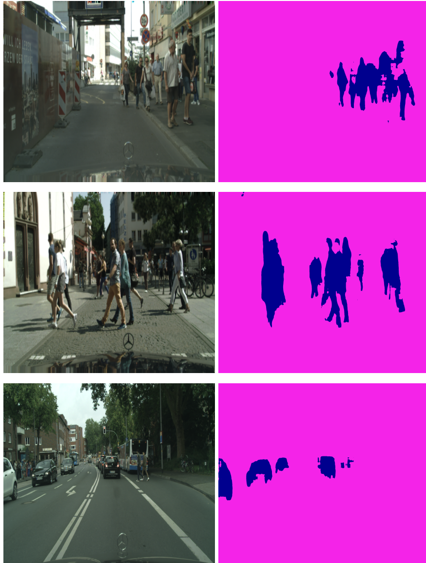
Fig. 2: Predictions of the modified lightweight BiSeNet model trained on Human Vs Non-Human and Vehicle Vs Non-Vehicle datasets.
